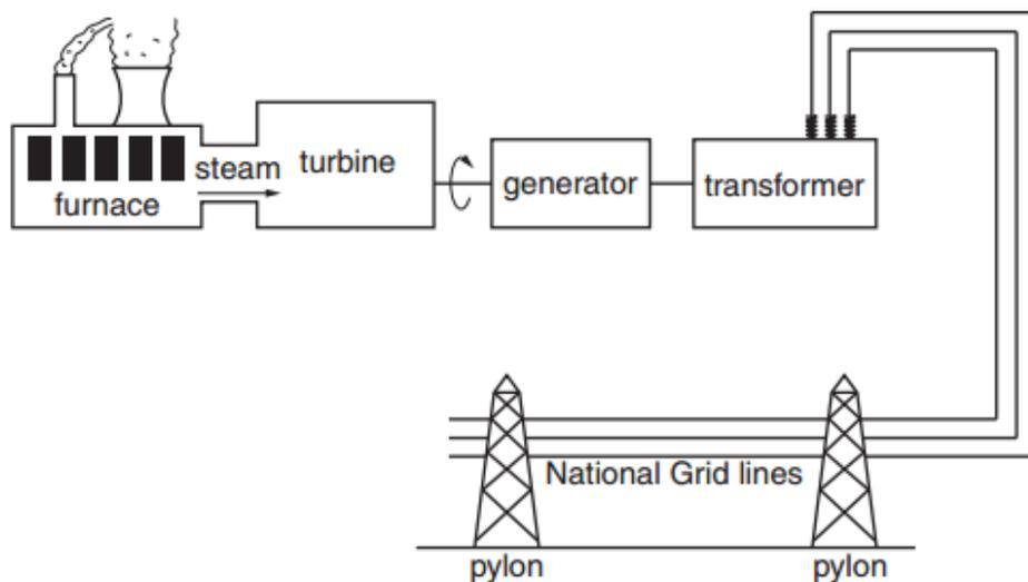
The generators in a power station produce alternating current (ac).
